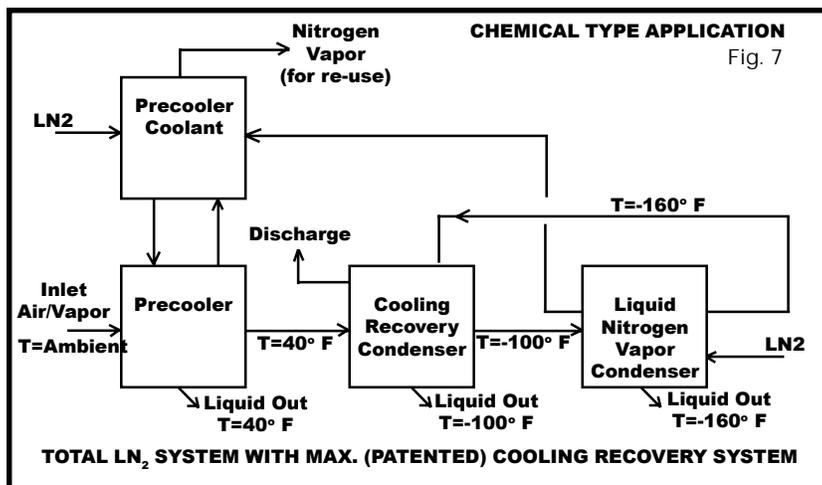
The units are sized for the maximum anticipated load and operate as required to maintain the design temperature in the condensing coils. When no vapor is being processed, the only operation is to maintain the coil temperature and the unit(s) will cycle off. This gives 0-100% turn-down ratio. This type of system ideally handles "spikes" typical in loading facilities and batch manufacturing processes.
