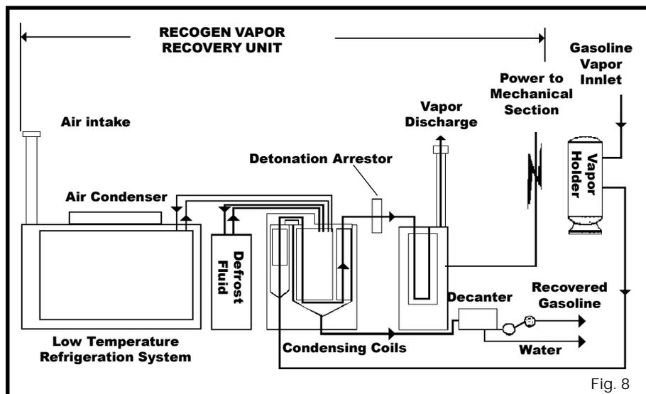
A standard range of RECOGEN units is available that meet the requirements of small, medium and large sized petroleum truck and marine loading terminals. Units can be provided that meet customer site specific requirements and comply with 40 CFR Parts 9 & 63 NESHAPS, 14 December 1994 as well as all current European Union and TA Luft standards. For gasoline vapor recovery, the standards are as follows:
